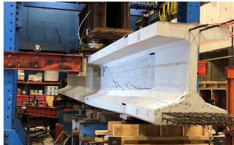
Fig. 17. Shear testing of a pretensioned UHPC bridge girder at the U.S. Federal Highway Administration. (Image by Benjamin Graybeal.)
